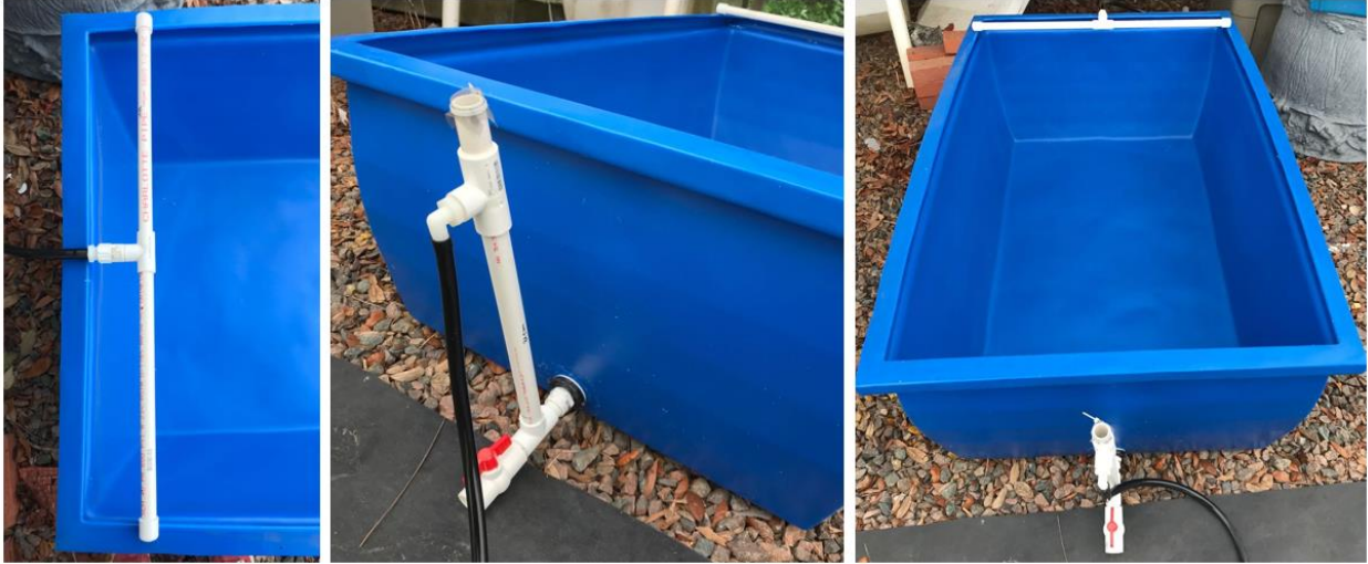
Figure 5: Photograph of HSSF-CW
