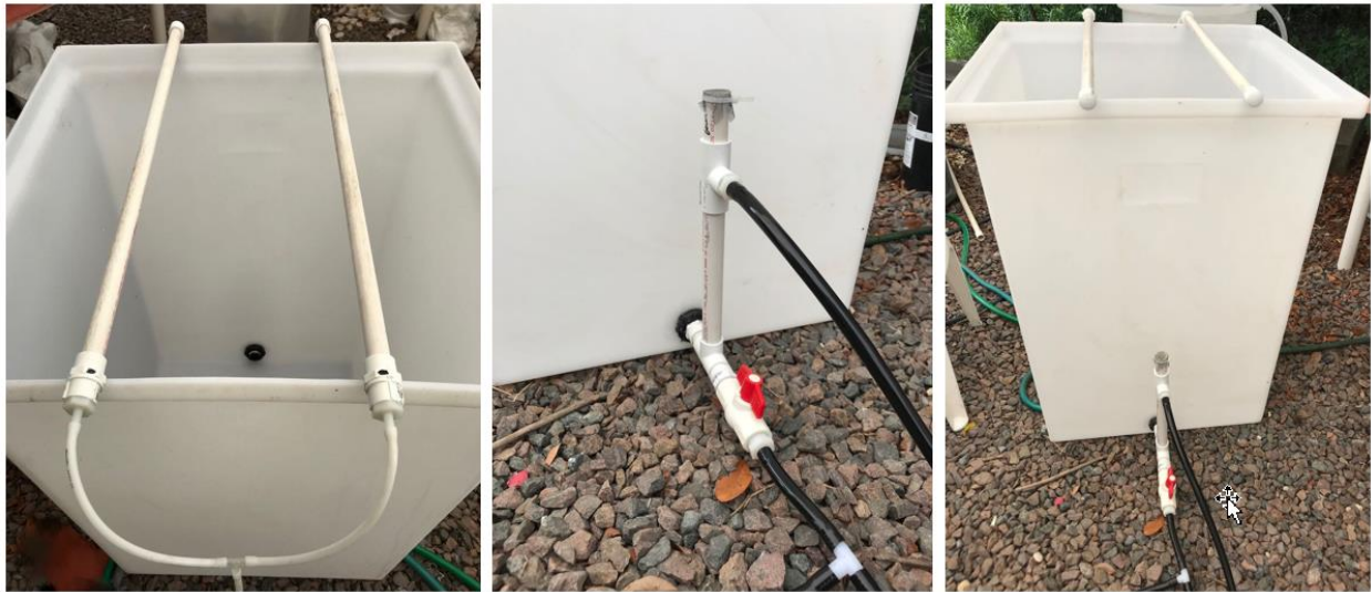
Figure 4: Photograph of VSSF-CW
